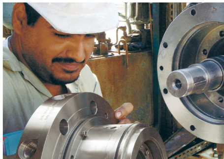
Dual mechanical seal EagleBurgmann SHV-D2/145-E1 installed at Saudi Aramco (Saudi Arabia) in a Sulzer helico axial multiphase pump. Operating conditions: t \dots 80\text{ °C} ( 176\text{ °F} ), p \dots 60\text{ bar} ( 870\text{ PSI} ), n \dots 4,000\text{ min}^{-1} .
