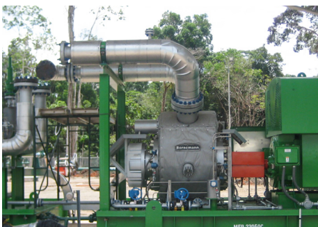
EagleBurgmann DFHSHJ4S1/110-E4 cartridge seal Operating conditions: t = \text{max. } 80\text{ °C} ( 176\text{ °F} ), p = 7\text{ bar} ( 102\text{ PSI} ), gas percentage ... 80 %. Medium: multiphase mixture, with 90 % water and gas.
